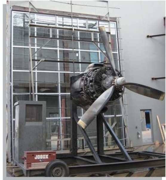
ATI Dynamic Pressure Water Test
